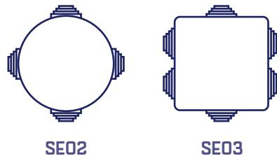
**SE02 & SE03** enclosures are supplied with pre-drilled 20mm<sup>2</sup> gland knockouts with soft rubber plugs that can be pierced for a cable to pass through, or removed if a separate cable gland is to be used.
